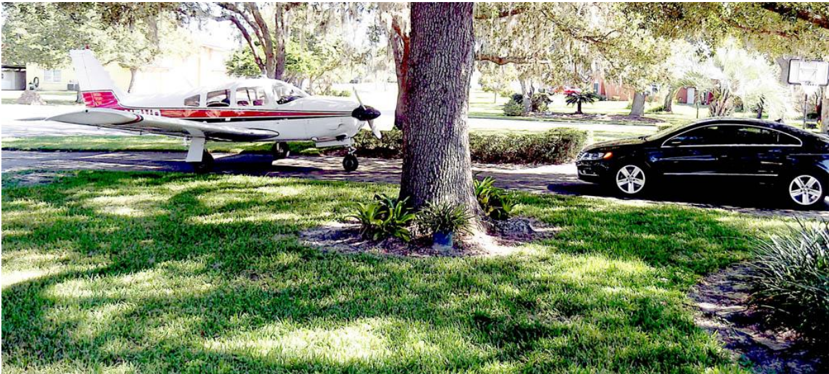
Photo 9: cars and planes share one access way to the residence. This saves money for the developer and allows greater use of the sealed road asset at airports that have low traffic flow.
